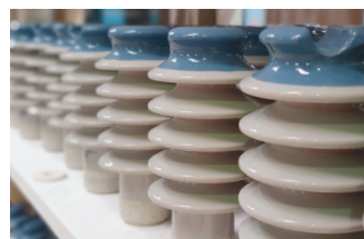
5. Fired 11kV insulators on a kiln truck.
