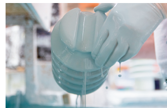
4. Glazing a post insulator (glazing forms a barrier to water ingress and gives strength to the insulator).
