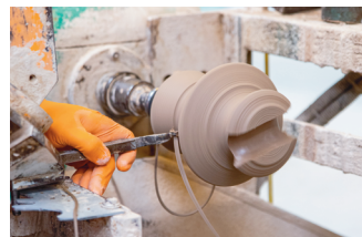
3. Turning (forming an insulator using a lathe) an 11kV Pin Insulator.
