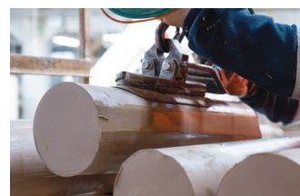
2. Clay blanks being loaded on to a stillage after undergoing the pugging process.
