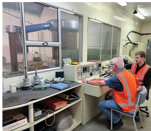
Rigorous electrical and mechanical testing is carried out at a safe distance on every NZI insulator
