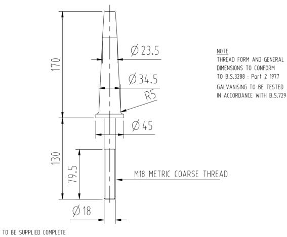
$\emptyset$  18.30  $\emptyset$  23.35 TOLERANCE ON THREAD FORM ± 0.1mm ( CHECK BY GAUGING )
